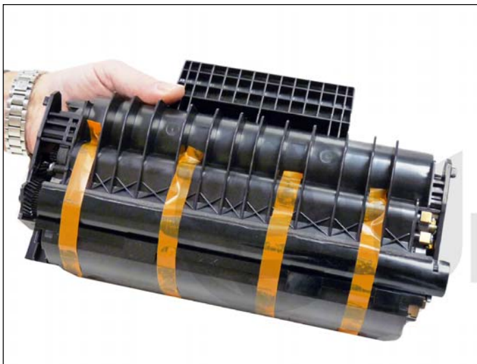
36. Install the drum cover if available. It needs to be taped in place. Use a brightly colored tape so the user will notice it.
