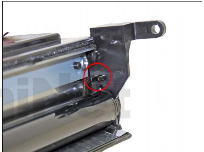
16. Remove the screw and holder from the gear side of the developer roller.
