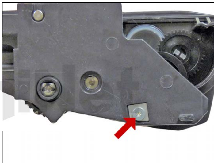
35. Install the metal plates and screws.
