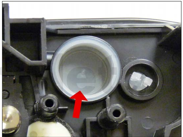
15. Remove the fill plug and dump out any remaining toner from the hopper.
