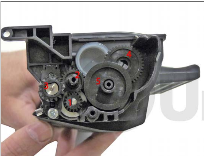
33. Replace all the gears on the hopper as shown.
